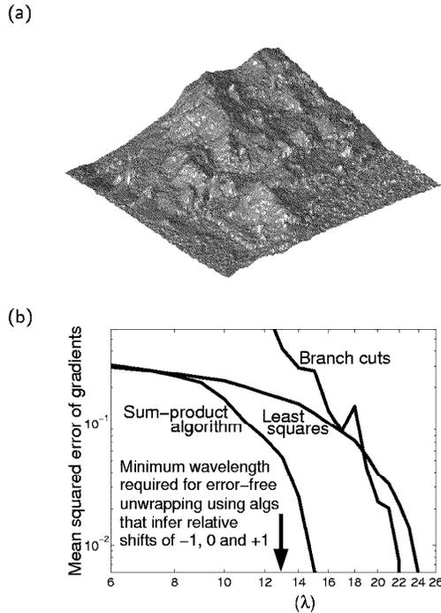
Figure 2: (a) After 10 iterations of sum-product algorithm on the wrapped map shown in Fig.1. Hard decisions were made for shift variables and the resulting gradients were integrated. (b) Comparison of performance of sum-product algorithm with other methods
