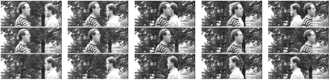
Figure 4: Three flexible sprites were learned from the input video (top row of frames), and then probabilistic inference was used to rerender the video frames, automatically removing various sprites.
