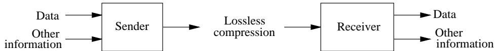
Figure 5: An illustration of how to make effective use of the freedom of choice available when there are several alternative ways of coding the data. Another source of information is used to decide between alternative codes. This allows the other information to be communicated as well as the data. So the true cost of communicating the data is reduced by the amount of information needed to choose between the alternative codes.
