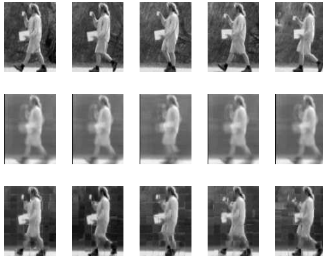
Fig. 6. (top row) Five images from an image sequence. (middle row) The single, large, six class TMG MAP approximation. (bottom row) The four class per grid cell TMG tree montage, MAP approximation.
